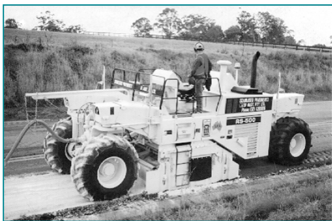
Fig. 2 Example of a Deep Lift Stabiliser (7)
